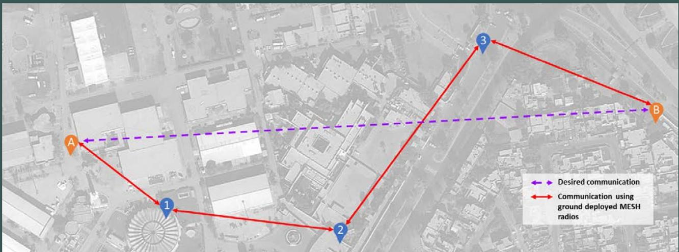
Communication needs to be established between point A and B but buildings are obstructing the line of sight. To overcome this problem, the MESH network utilizes other ground deployed radios. However, this solution is not optimal as it depends on having sufficient ground radios deployed at the right place at the right time or by having a number of MESH radios installed in strategic locations. Neither of these approaches are fast, flexible or simple to deploy in a complex environment.
